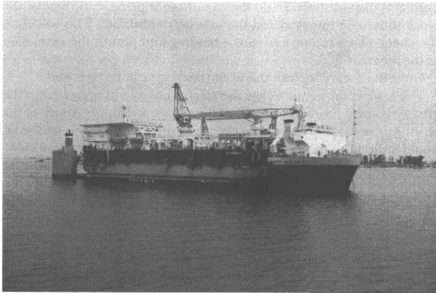
The heavy lift vessel 'Sea Servant 3' engaged in the transport of the crane barge, 'Al-Baraka 1'.
