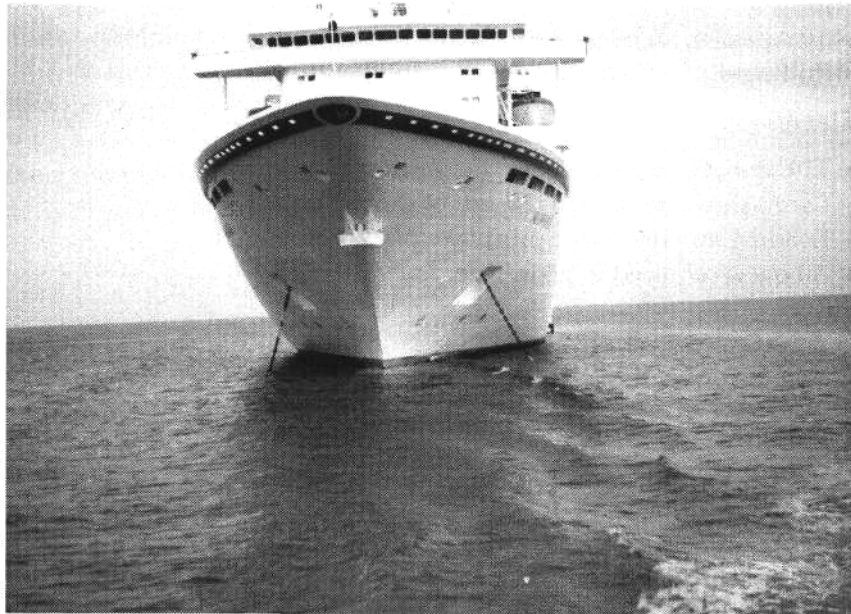
The 'Seaward', Class 1, passenger cruise ship, seen moored at anchor with both port and starboard anchors deployed.
