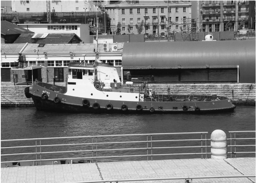
Harbour Tractor Tugs. An example of a large harbour tug, laying starboard side to the berth in Lisbon, Portugal. Tugs tend to be well fendered, all round, with a bow pudding fender arrangement which permits pushing as well as pulling. A towing hook arrangement is situated just aft of the amidships position, aft of the accommodation block.
