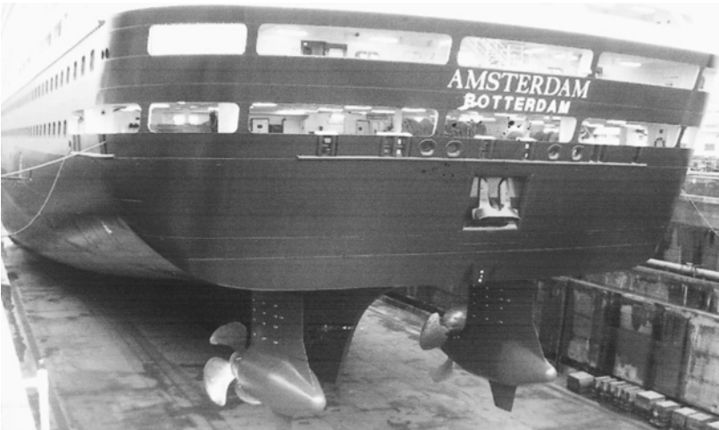
The Passenger vessel 'Amsterdam' fitted with twin azipod propeller units either side of the centre 'skeg', seen exposed in the dry dock environment. Alternative arrangements are constructed with a centre line Controllable Pitch Propeller with azipods set to either side.
