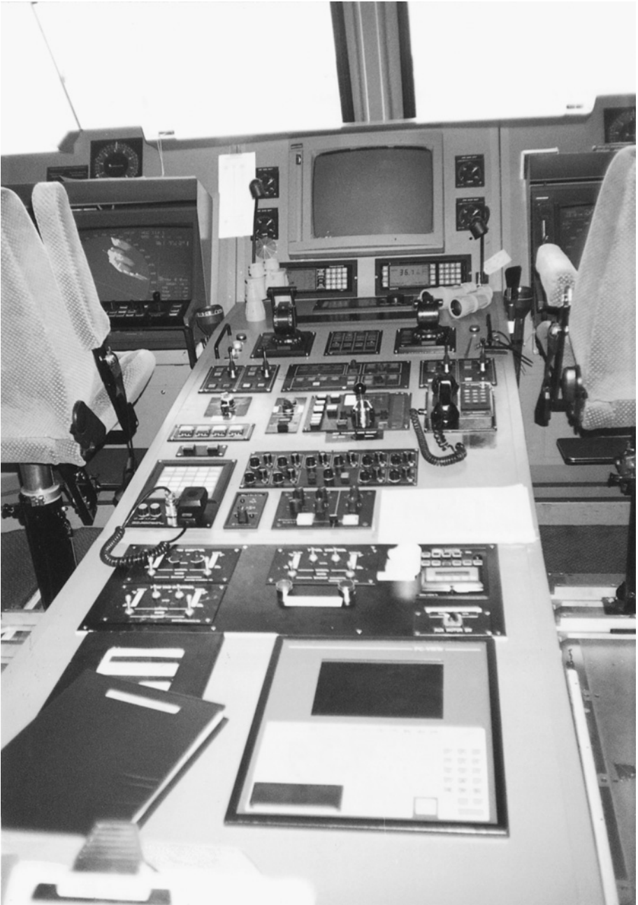
High speed craft – bridge consol. A typical central position, bridge consol for a modern high speed ferry craft. Interchangeable LCD monitors for ARPA and ECDIS displays are set either side of manoeuvring controls and the centre performance and status data display.
