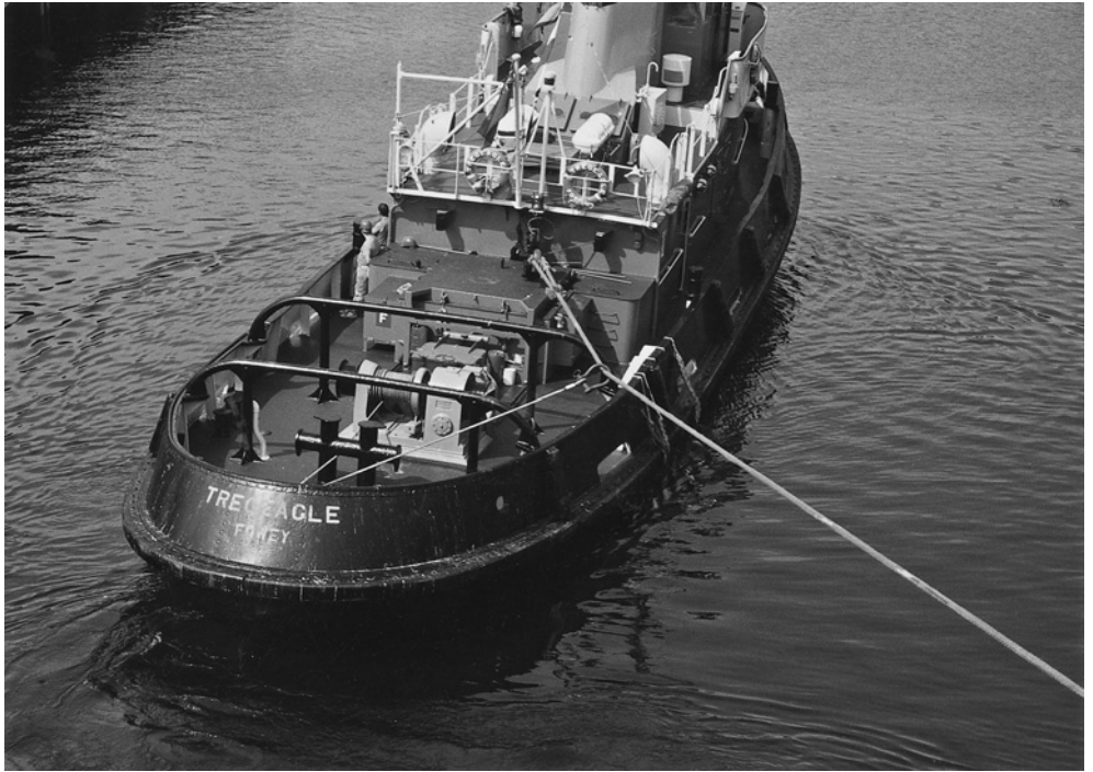
Control of wire towing line by means of gob wire and heavy duty shackle.
