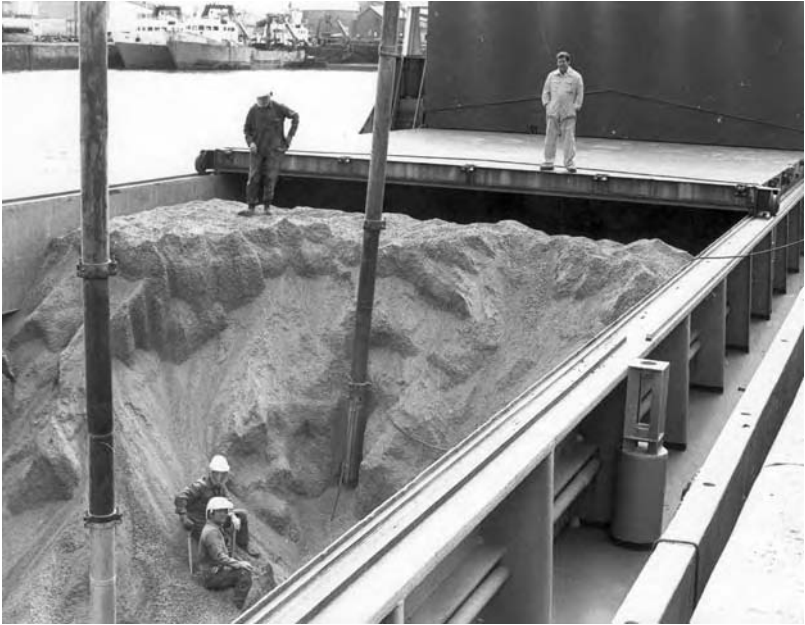
Fig. 4.11 Discharge of grain/cereals. The suckers from 'grain elevators' discharge cereals contained in a ships bulk cargo hold from under the rolled back steel hatch covers. Men in the hold actively use the heel ropes to drag the suction into areas of cereal concentration.
