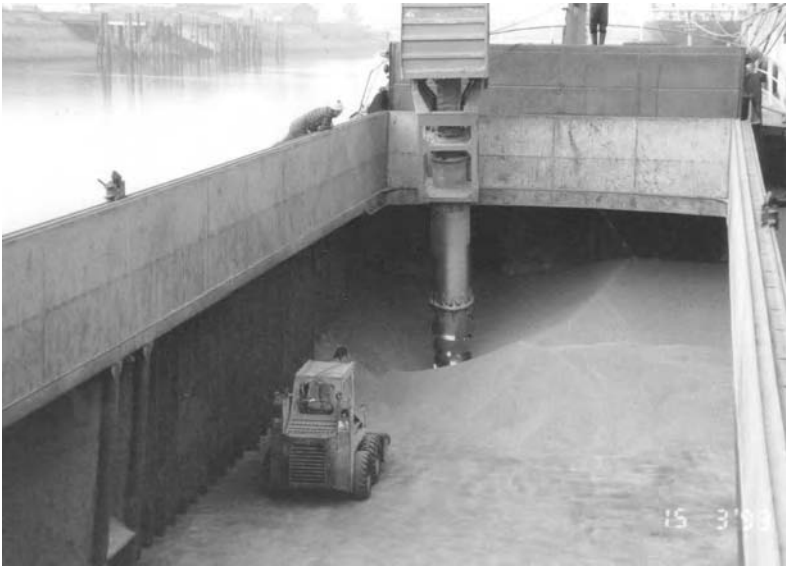
Fig. 4.13 A tractor is engaged in the tween deck of a vessel discharging cereals, to ensure that the suction of the grain elevator has access to all residuals of the cargo product.
