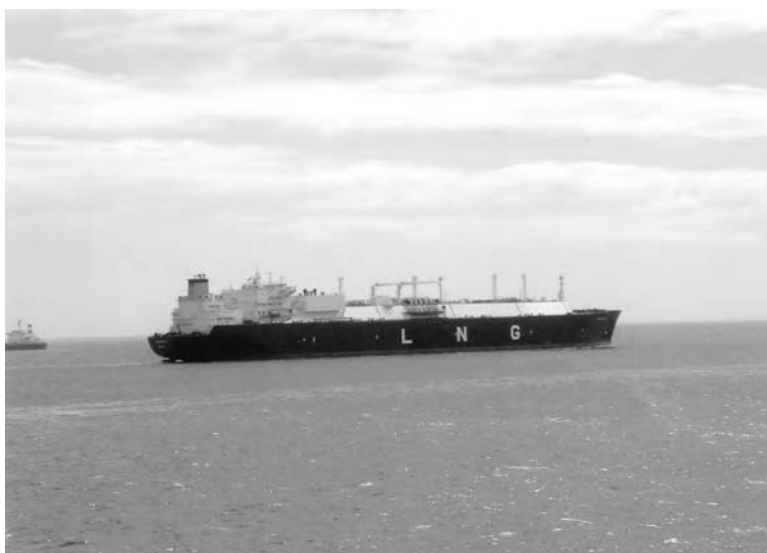
Fig. 5.30 LNG carrier. Profile of an LNG vessel seen lying at anchor off Gibraltar harbour. Prismatic tank design as opposed to the spherical tanks.
