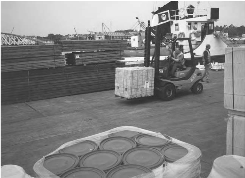
Fig. 1.22 A fork lift truck operates case goods, stacked timber parcels and palletized drums on the quayside for general cargo vessels.
