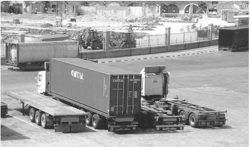
Fig. 7.18 Ro-Ro, unit types. Several Ro-Ro units on the quayside in Cadiz, Spain. From left to right: a flat-top trailer unit, a 40-ft container carrier, with two articulated container carriers on the end. A mobile tank container trailer unit is seen in the background.
