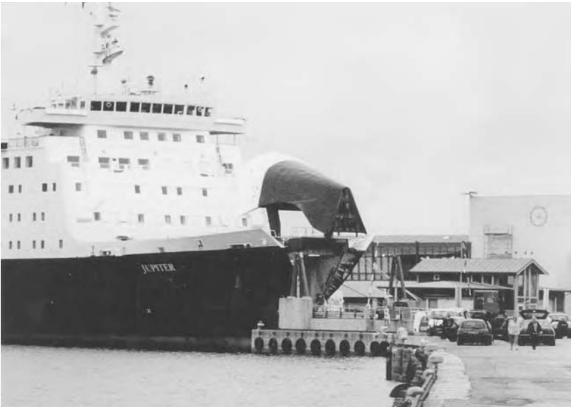
Fig. 7.7 The bow visor of the passenger vessel 'Jupiter' (since renamed) seen in the open position against the skyline. The bow visor fitted with a stern ramp access permits a drive through capability.
