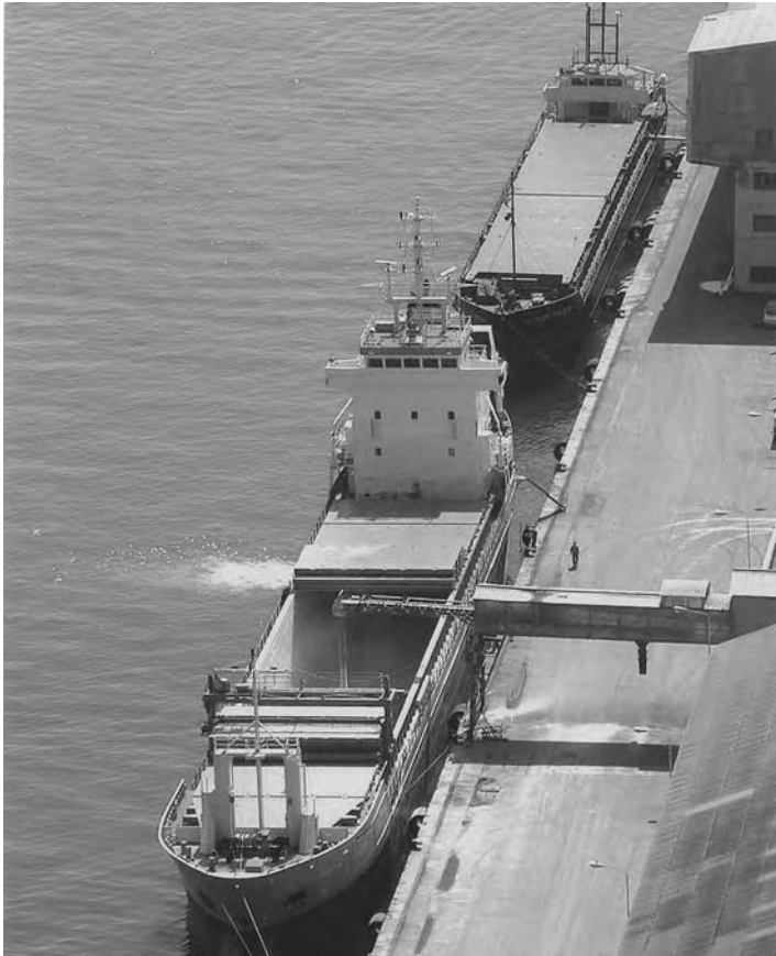
Fig. 2.12 Two bulk carrying 'feeder' coasting vessels lie port side to, alongside the grain elevator in Barcelona. The lead ship is seen discharging with partially opened steel hatches, operated by its own mini-gantry crane. The one astern has folding weather deck hatches in the closed-up position.
