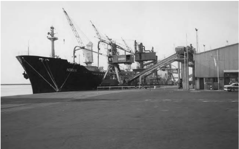
Fig. 1.14 The 'Norvik' general cargo vessel pictured in the Port of Limassol, Cyprus. The ship has turned her deck cranes outboard to allow access for the suctions of the grain elevators to discharge a bulk cargo of grain.
