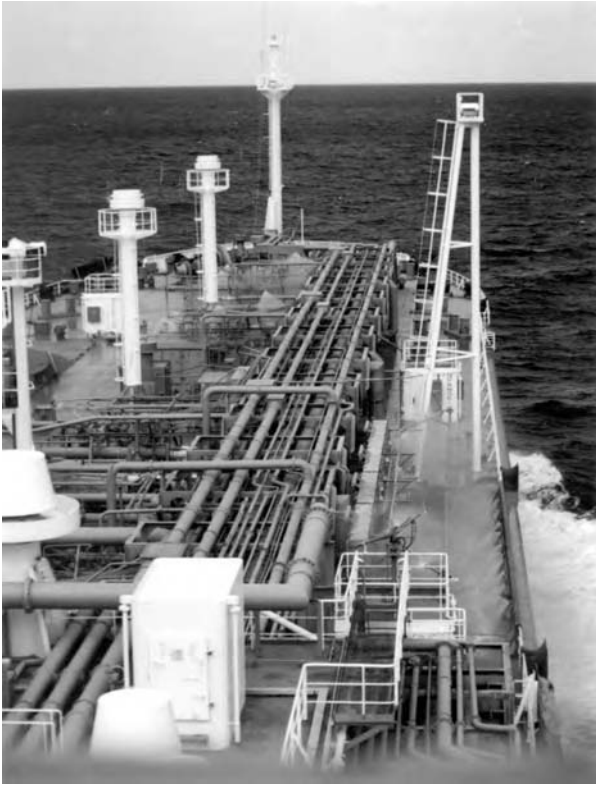
Fig. 5.9 Tanker deck arrangement. Typical example of the pipeline (fore deck) arrangement of a medium size oil tanker seen in the sea-going environment.
