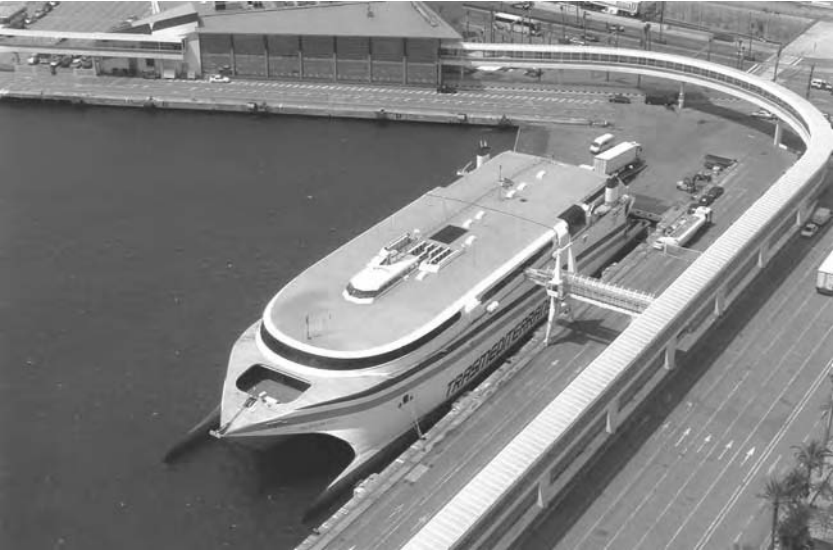
Fig. 7.25 The high-speed Ro-Pax catamaran vessel 'Millenium Dos' seen loading vehicles via the stern access, lying port side to the terminal in Barcelona, Spain.
