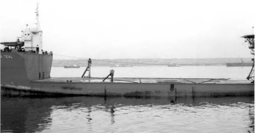
Fig. 2.26 The steel deck space of the 'Sea Teal' a heavy-lift transport. The tank ballast system, allows the deck to be submerged to allow a Float-On, Float-Off, system to take place for heavy-lift or project-cargoes.
