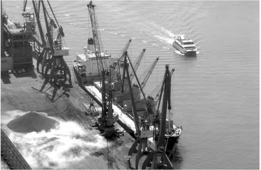
Fig. 4.2 An overhead view of a general cargo vessel engaged in the discharge of concentrates by means of a free-standing crane using a mechanical grab. The ship's own deck cranes are turned outboard to allow easy access for the shoreside crane operation.
