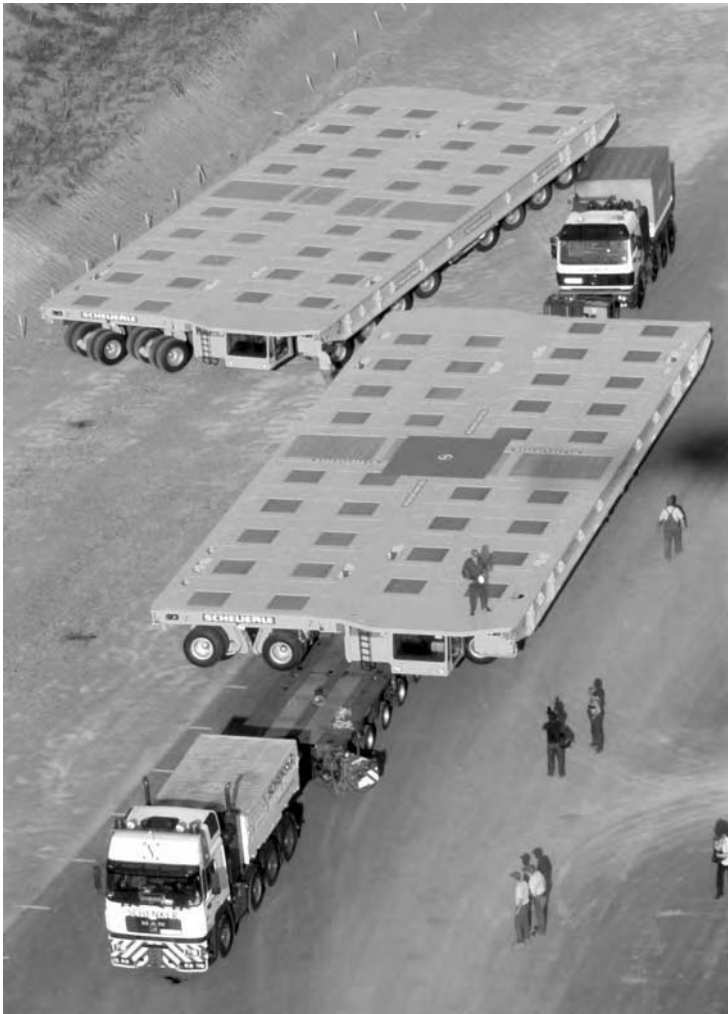
Fig. 2.31 Multi-wheel heavy load transports. Manufactured by the Scheuerle Company of Germany. The mobile platforms provide multi-axle transport for the large heavy load and are regularly inter-connected for the project load carrying up to 10 000 tonnes. Variations for smaller loads range from the 15-tonne low-bed trailers to platform trailers of up to 1000 tonnes.
