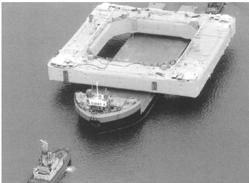
Fig. 2.29 Project type cargoes. The Smit 'Giant 4' heavy-lift transport engages with a 6500-tonne lift, designated for the 'Visund Field' offshore. Giant 4, is a 24 000 dwt submersible heavy duty transport barge. The operation was conducted by a Load-out/Float-off arrangement in June 1997.
