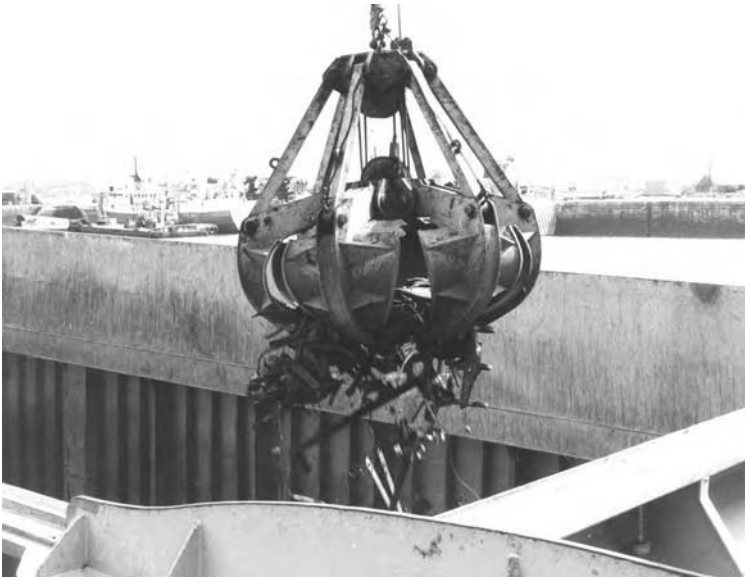
Fig. 4.3 Working bulk cargoes. Mechanical grabs discharging 'scrap metal' from the cargo hold of a small bulk carrier. The single hull construction shows the athwartships, side framing, positioned vertically below the hatch coaming.
