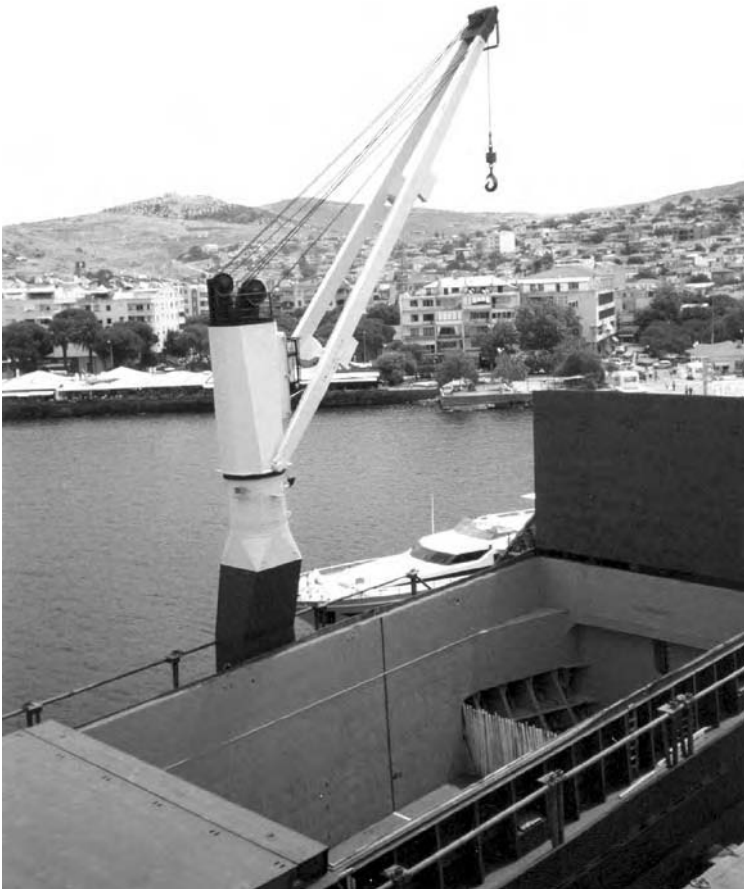
Fig. 1.11 Example of a Deck 25 tonne SWL crane aboard the general cargo vessel Scandia Spirit. The vessel carries two deck cranes, both mounted on the port side of the vessel.
