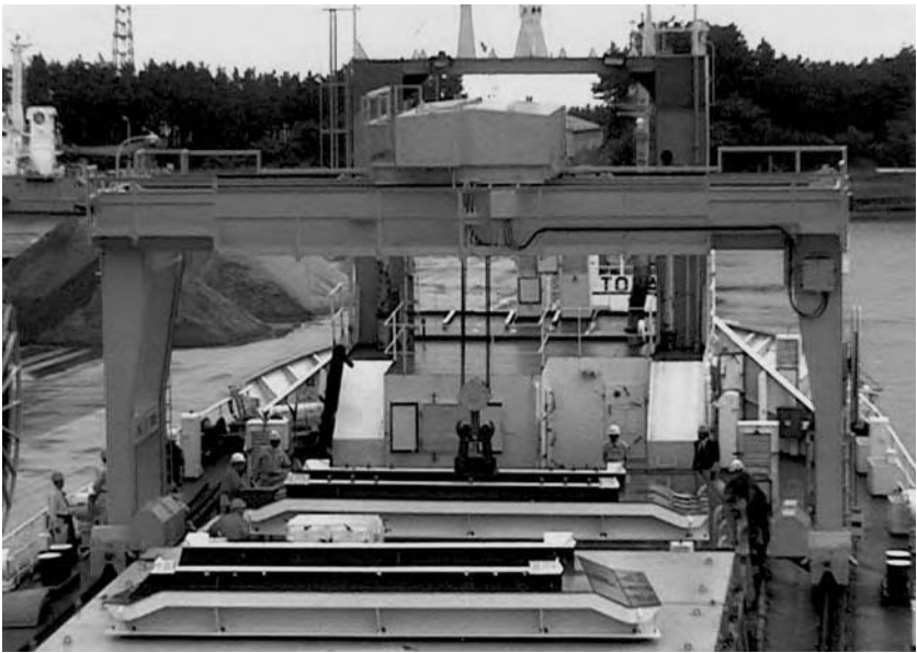
Fig. 1.15 Example of a mobile tracked gantry crane in operation on the ships foredeck. Suitable for a vessel with all aft accommodation.
