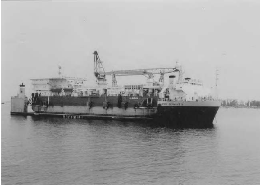
Fig. 2.27 The heavy-lift vessel ‘Super Servant 3’ seen loaded with the crane barge AL-Baraka 1, lies at anchor awaiting to discharge its load by Float-off methods.
