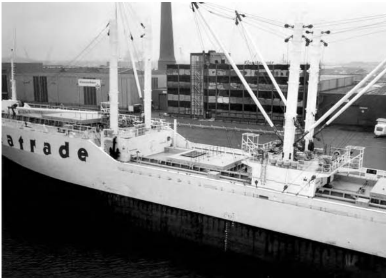
Fig. 1.3 The conventional derrick rig. Modern general cargo vessel rigged with conventional 5 tonne SWL derricks and steel hatch covers. The derricks can be rigged to operate as single swinging derricks or rigged in 'Union Purchase' SWL (U) = 1.6 tonnes. Such vessels are in decline because of the growth in unit load 'Container and Ro-Ro, Traffic'.
