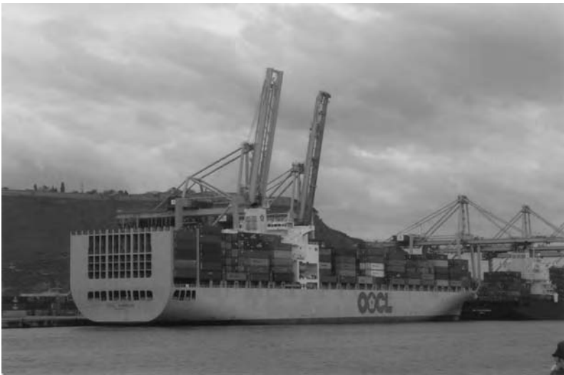
Fig. 8.13 The 'OOCL Shanghai' lies port side to the container terminal in Barcelona, Spain, after completing cargo loading with a full container load, the deck stack being at a six-tier height. The terminal 'gantry cranes' seen in the upright and clear position (the ship is not fitted with its own crane).
