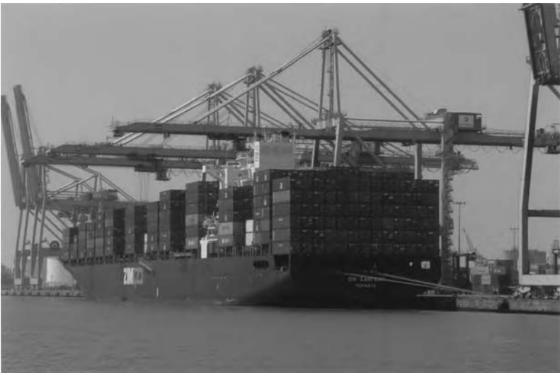
Fig. 8.3 The container stack on the deck of the 'ZIM ΣANIKAH' being discharged by terminal 'gantry cranes' in the Port of Barcelona, Spain.
