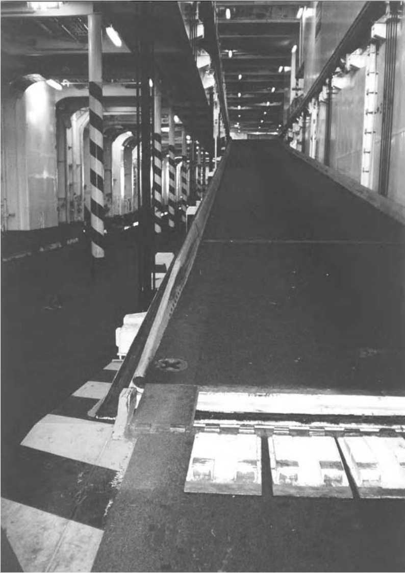
Fig. 7.12 An internal ramp that can tilt both forward and aft to suit stern load and/or bow discharge. It allows loading to a higher deck level 'three' where the lower hold level would be termed 'No. 1 Deck Level' and 'No. 2 Deck Level' would be considered as the main, largest of the three vehicle decks.
