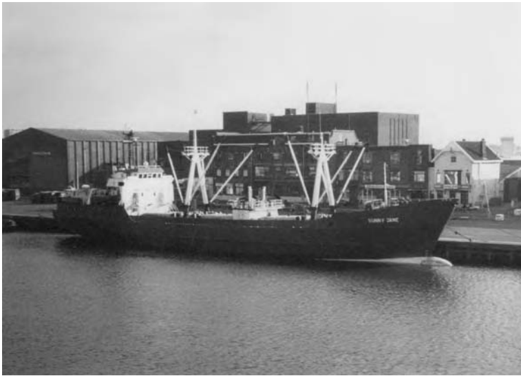
Fig. 1.1 The conventional 'general cargo' vessel 'Sunny Jane' lies port side to, alongside in the Port of Amsterdam. The vessel is fitted with conventional derricks, supported by bi-pod mast structures.
