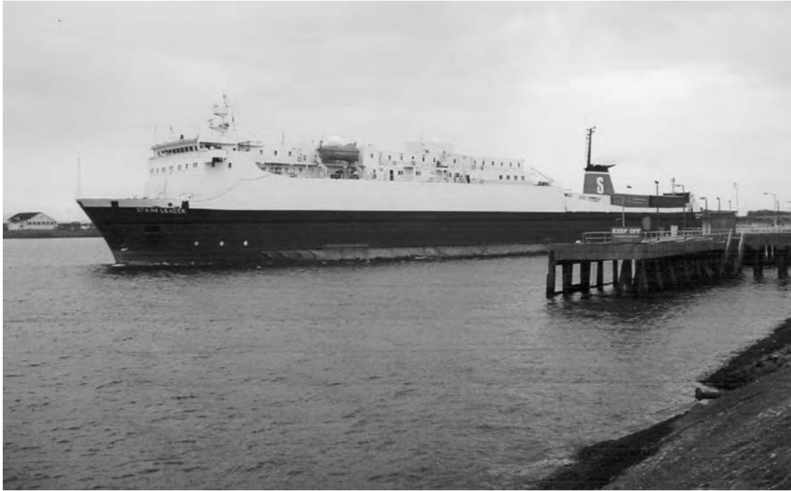
Fig. 7.1 Ro-Ro shipping. A typical Ro-Ro ferry the 'Stena Leader' (previously European Leader and ex-Buffalo, P&O Ferries) departs the Port of Fleetwood for her regular twice-daily voyage to Ireland. The vessel carries about 140 mobile units (40-ft container size) on three vehicle decks. The ship also accommodates a limited number of unit drivers.
