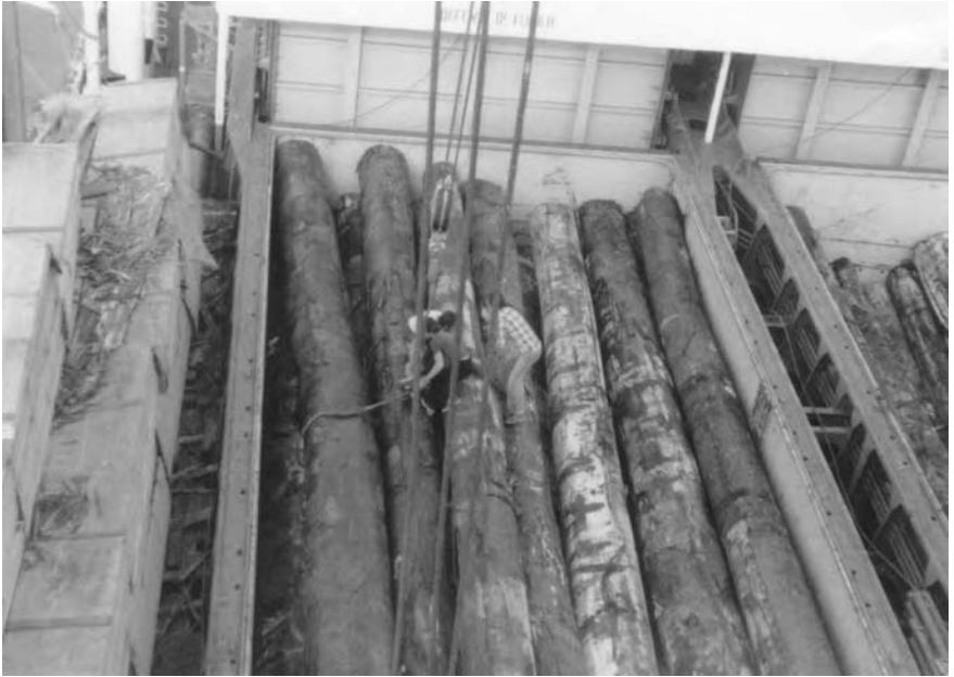
Fig. 6.5 Stowage and the Working of Timber Cargoes. A cargo of logs stowed underdecks in twin hatches, being discharged by multi-fold lifting purchase. Wire snotters are used to manoeuvre the logs to allow slings to be passed under, prior to discharging. Slings are often left in situ after loading to ease discharge but not always. Sawn bundles of lumber are seen stowed at the hatch side as deck cargo.
