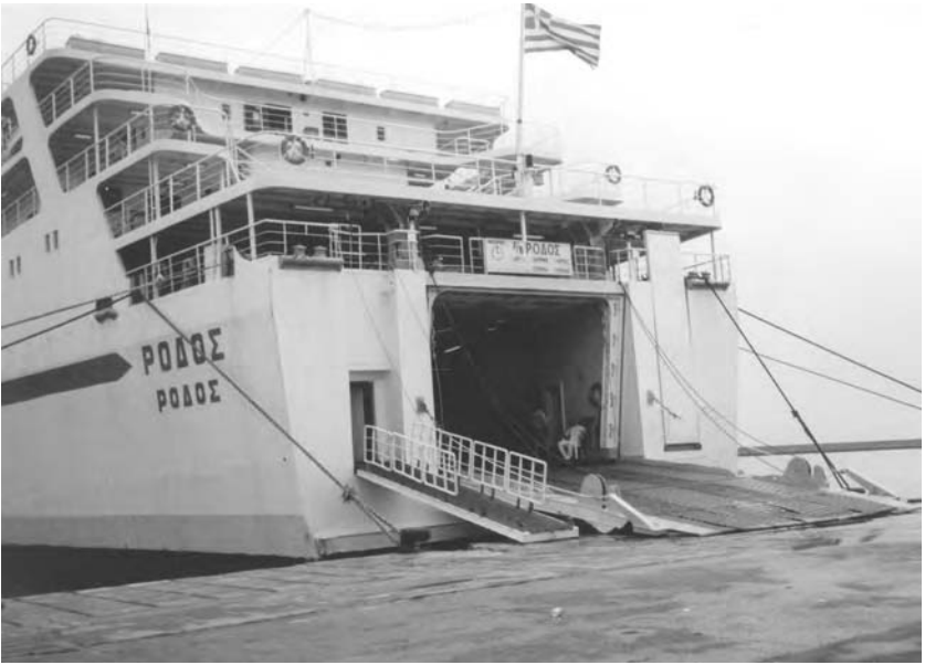
Fig. 7.6 Ro-Ro ferry example. Stern door/ramp access into the enclosed vehicle deck of a Ro-Pax ferry operating in the Mediterranean Sea.
