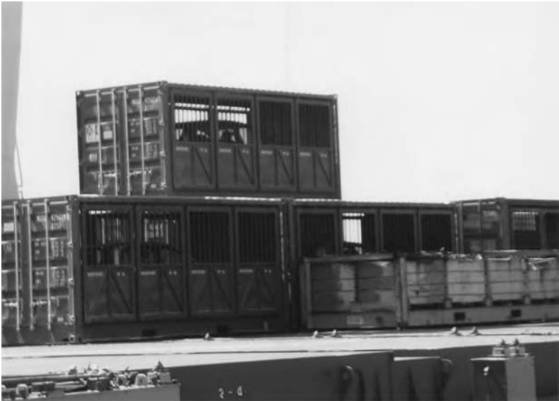
Fig. 8.18 Part loaded deck of the vessel 'Hydra J'. Containerized vehicles and half-height container seen clear of securings and ready for discharge.
