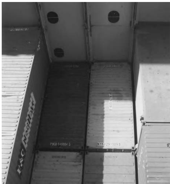
Fig. 8.14 Container (internal) hatch stowage. Container hatch with part load containers lying in the cell guides of the lower hold cargo space.
