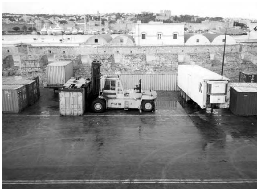
Fig. 1.23 Ground handling of large loads, like containers, can also be achieved by using the larger, high capacity 'fork lift' trucks on the quay side. Expansion forks of extended length are used for wide loads up to about 12 tonnes.
