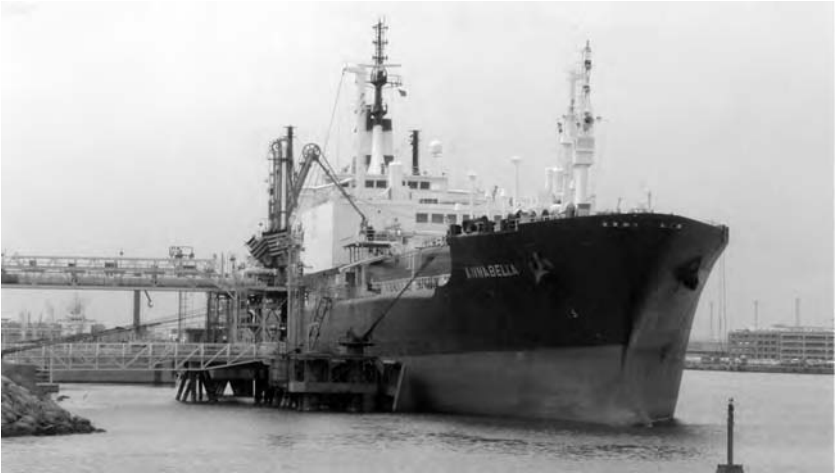
Fig. 5.31 The Monrovia Gas Tanker 'Annabella' seen starboard side to the Gas Terminal in Barcelona while engaged in gas cargo operations.
