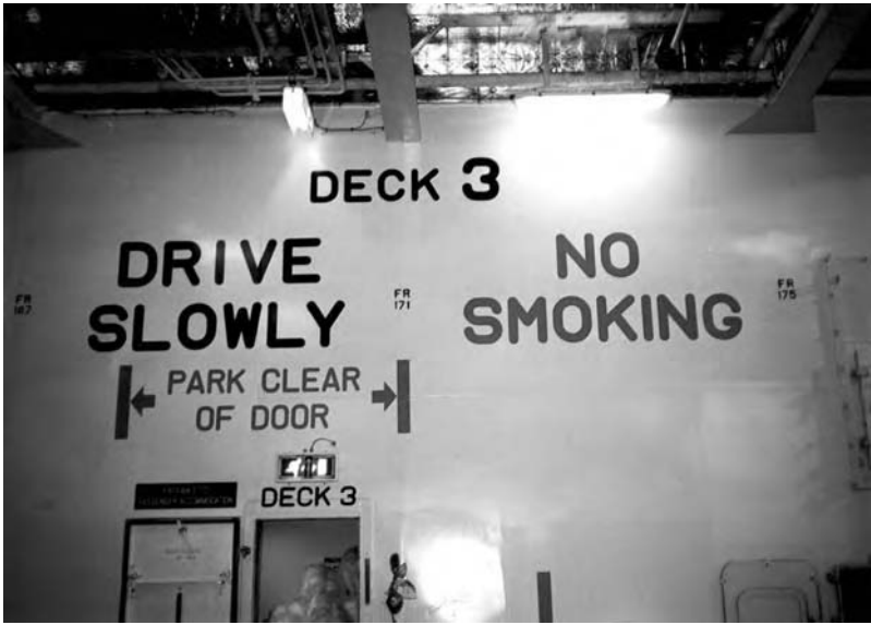
Fig. 7.15 Typical bulkhead markings prominently displayed around vehicle decks to ensure safe and efficient loading of vehicle lanes.
