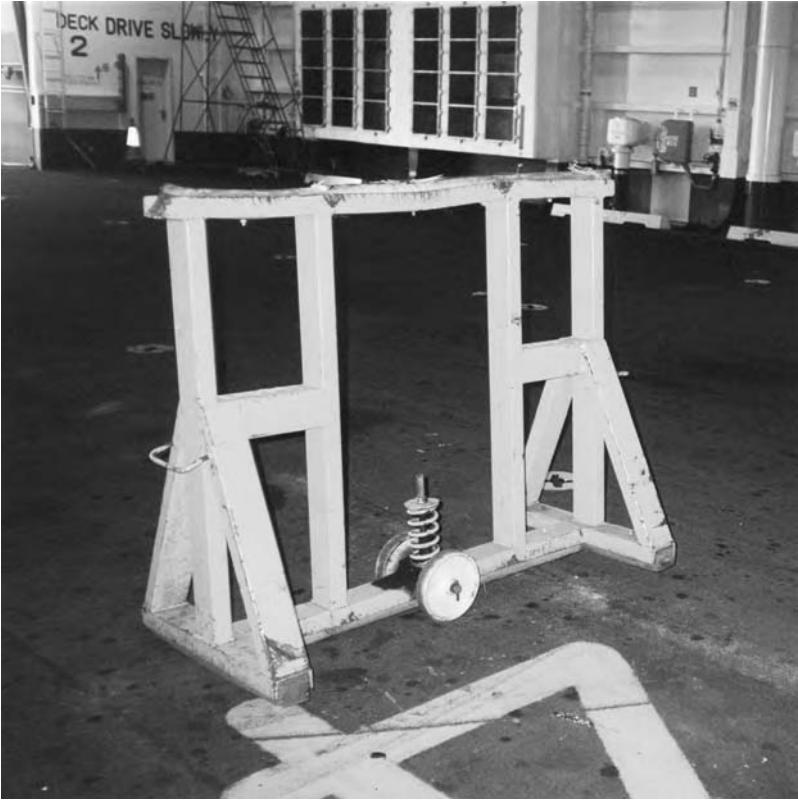
Fig. 7.21 Wheeled trestle is positioned under the unit before being detached from the motor tug. Trestles fitted with spring-loaded wheels to permit easy manoeuvring under the cargo unit.
