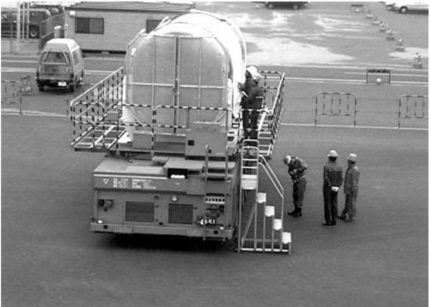
Fig. 10.2 Security personnel monitor nuclear waste flasks, following discharge into the port facility handling grounds. Customized transports are designated to each flask and movement is checked at every stage of transit.
