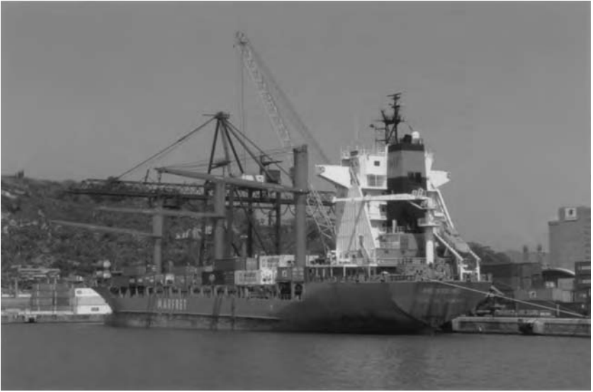
Fig. 8.27 A single gantry crane and a mobile dock side crane work the container cargo of the feeder container vessel 'Providence'. The ship's own container cranes are seen turned outboard to facilitate the shoreside loading systems in the port of Barcelona.
