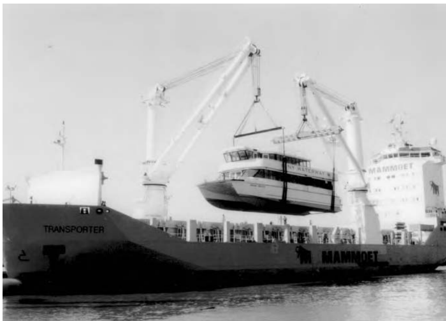
Fig. 2.20 The 'Transporter' of the Mammoet Shipping Company is seen engaged in the lifting of a ferry vessel destined for the New York Waterway system. The lift is being made by means of two heavy-duty ships 'Huisman' cranes, each of 275-tonne SWL. The tandem lift takes place using lifting beams having a capacity of up to 250-tonne SWL.
