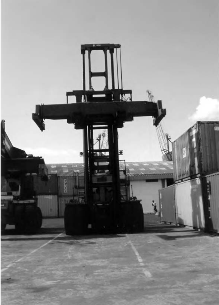
Fig. 8.35 Container terminal movement. Container transporter, with lift, transport, and stacking capability. A type of container karrilift based on the fork lift truck principle which is widely employed in container terminals worldwide.
