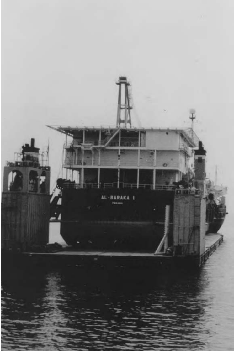
Fig. 2.28 Stern view of the heavy-lift vessel 'Super Servant 3' with the crane barge load seen in the Arabian Gulf area.
