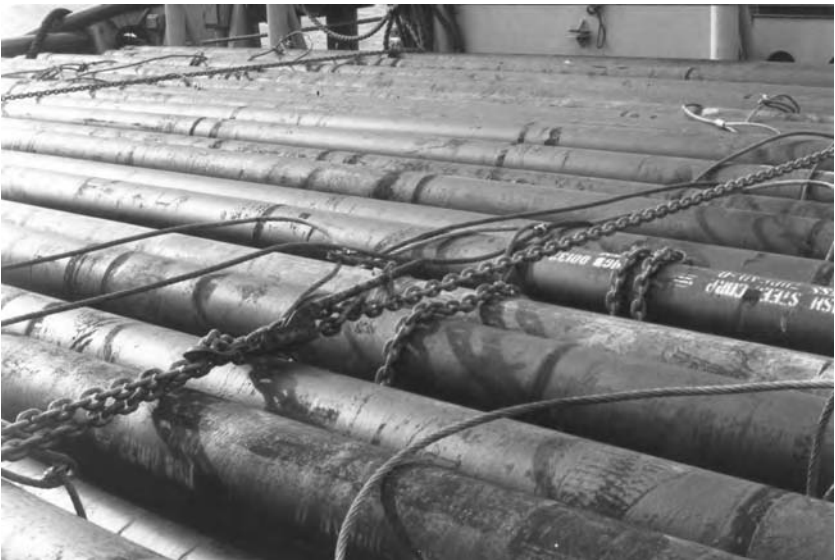
Fig. 9.3 Securing deck cargoes. Steel pipes seen stowed on upper decks. Chain lashings are stretched across at intermediate lengths and tensioned by ratchet gear once in position. The pipes have been left pre-slung with wire snotters for speed of discharge.
