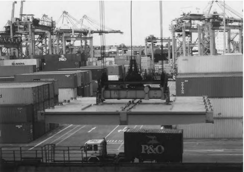
Fig. 8.23 The container hoist engaged in lifting the pontoon hatch covers clear of the cellular holds.
