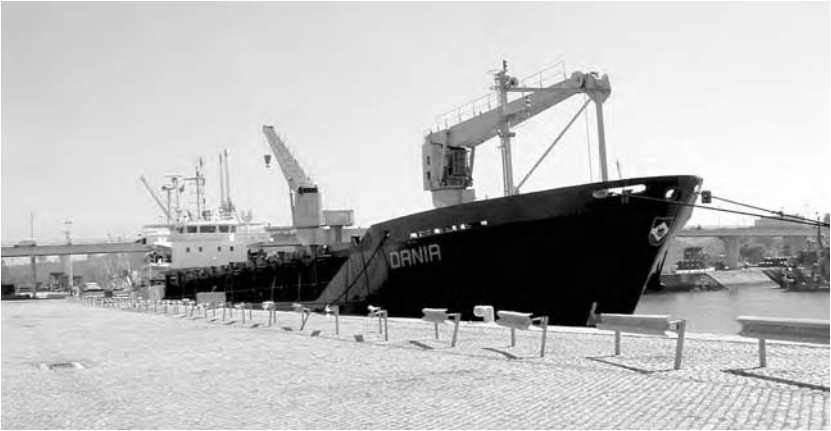
Fig. 1.13 The two deck cranes of the 'Dania' a general cargo/heavy-lift/container option vessel seen lying starboard side to, in Cadiz, Spain. The aft crane is seen in the elevated position while the forward crane is in its stowed position (SWL = 35 tonnes).
