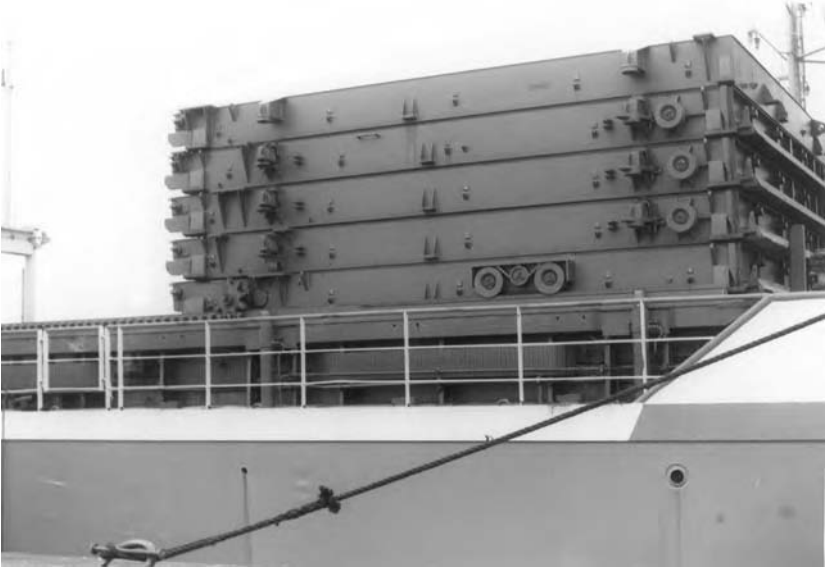
Fig. 2.6 Rack and pinion horizontal stacking steel hatch covers seen in the hatch open position. The drive chain running the length of the hatch tracks.
