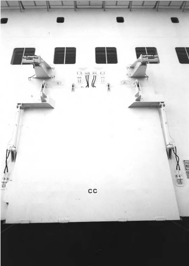
Fig. 7.13 Cargo doors. Upper deck hydraulic cargo door set in the bridge front and leading to an enclosed upper vehicle deck aboard a modern Ro-Pax ferry. Weather sealing of the door takes place against hard rubber seals with hydraulic cleating and positive pressure held on operational rams. When in the open position the door is locked with hydraulic securings and rams are fitted with non-return valves to prevent accidental closing.
