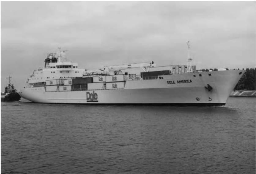
Fig. 8.7 The 'Dole America' container vessel manoeuvres with tugs in attendance inside harbour waters. Containers are stacked two high on deck and the two ships container cranes are seen in the stowed, fore and aft position.
