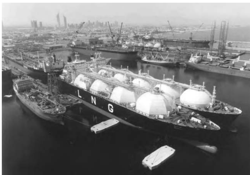
Fig. 5.26 Two LNG carriers lie alongside each other outside the Dubai Dry Dock Complex. These dedicated ships are prominent by the conspicuous cargo domes covering the gas tanks.
