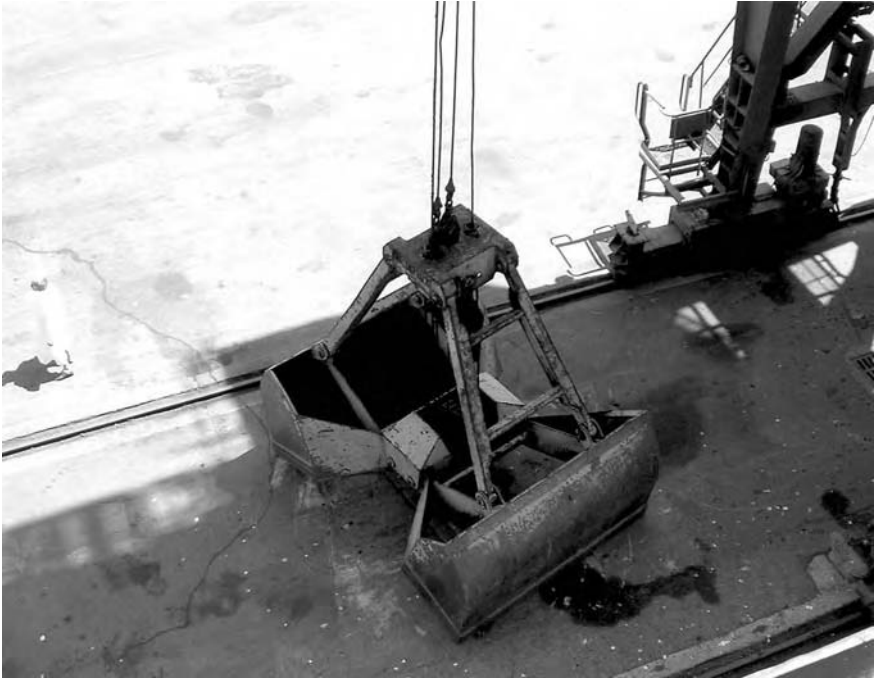
Fig. 4.14 Bucket mechanical grab seen in the open position on the quayside. The crane is configured so that the controlling crane driver can open and shut the grab by means of an operational wire to open and close the bucket arrangement.
