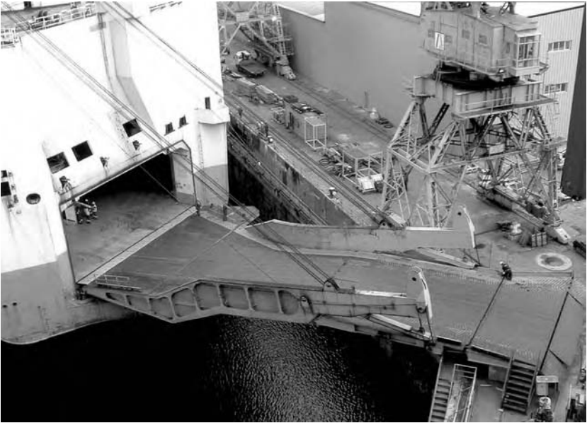
Fig. 7.30 A specialist unit load system. The angled quarter ramp and access point to vehicle decks of the above car carrier. These angled ramps have become a popular feature of car carrier vessels and are often employed with a midsection shell door ramp to improve the speed of load and discharge operations.
