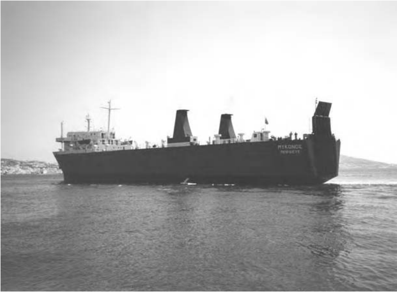
Fig. 7.4 Modern Ro-Ro (freight only) vessel. The 'MYKONOS' a modern Greek operated Ro-Ro vehicle ferry. Design features include all accommodation forward, with twin Port and Starboard smoke stacks seen aft either side of the upper vehicle deck. The stern door/combined vehicle ramp is positioned right aft in the upright closed position while the vessel is at sea.
