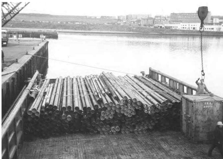
Fig. 9.4 Capped drilling pipes seen loaded on the wide beam cargo deck of an offshore supply vessel. The pipes are capped at each end to prevent water retention in the event of the vessel encountering rough weather. Any fluid in quantity being retained amongst deck cargoes could seriously affect the positive stability of the vessel.
