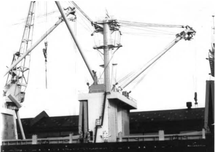
Fig. 1.10 Speed crane/derricks in operation from on top of the Mast House of a general cargo vessel.
