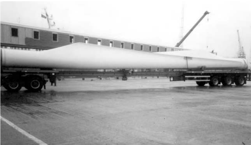
Fig. 7.17 Long load (sail for wind turbine) is loaded on adjustable stretch load trailer unit.
