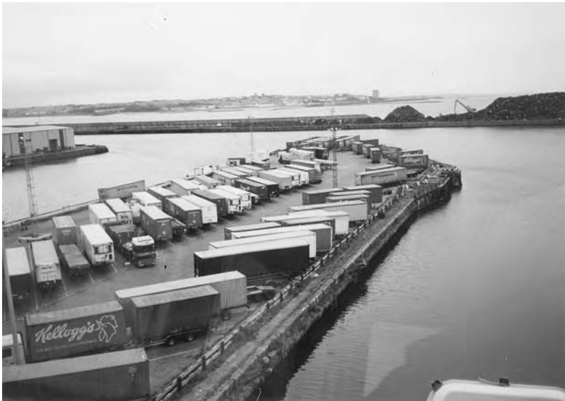
Fig. 7.16 Ro-Ro traffic trailer units, parked on the dock side at Liverpool ready for loading on to P&O, Irish sea ferries. Trailer units being lifted by mechanical 'tugs' and deposited on the vehicle decks of short sea ferries then similar 'tugs' attach to discharge the unit at the destination port.
