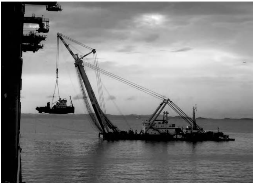
Fig. 2.24 The Smit 'Cyclone' floating sheer leg barge, engages in a general cargo heavy-lift operation on the vessels offshore side.
