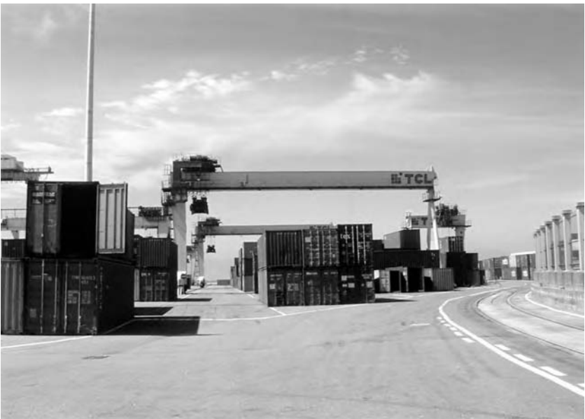
Fig. 8.30 Tracked, terminal stacking gantry cranes operate through the Lisbon container terminal. Rail and road park transport having access to the container park.
