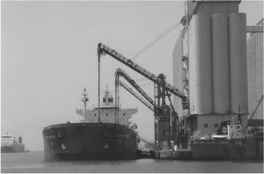
Fig. 4.10 The bulk carrier 'Alpha Afovos' lies port side to the grain silos in Barcelona. The grain elevators seen deployed into the ships hold effecting discharge.
