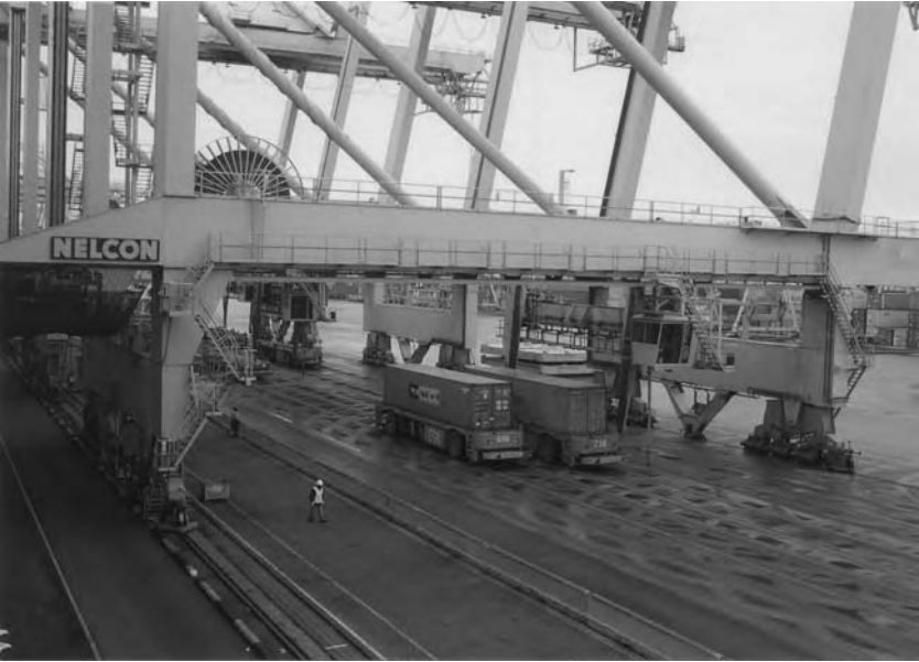
Fig. 8.24 Tracked shoreside 'gantry crane' for the loading of containers, semi-automatic, driverless transports deliver containers to its underside for loading aboard the container vessel.
