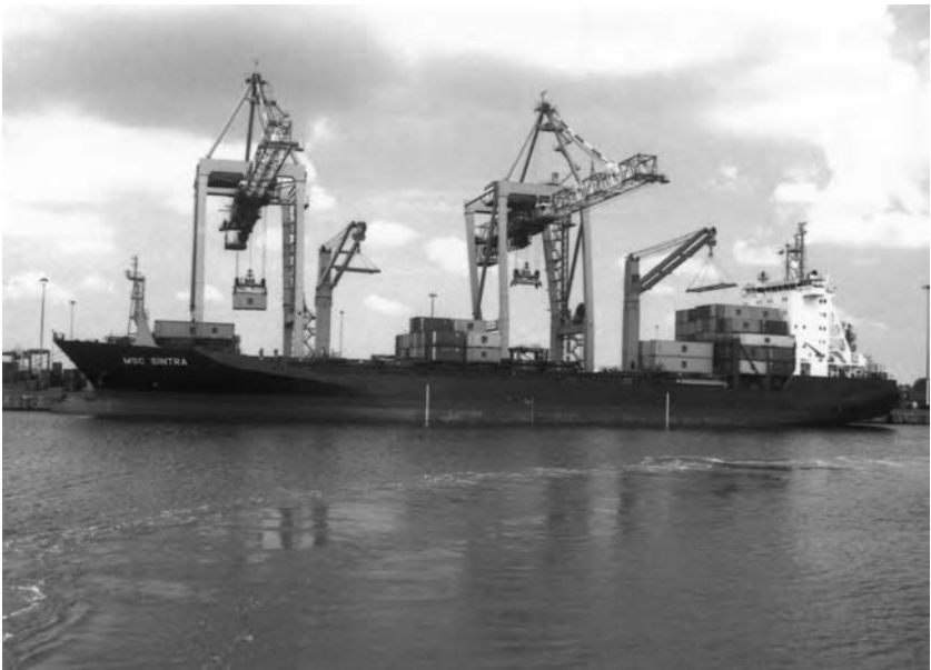
Fig. 8.4 Working containers. The Mediterranean Shipping Company (MSC) Sintra lies starboard side to working containers by shoreside gantries in St John's, Newfoundland container terminal. The ship's own two container cranes are turned outboard to permit access by the gantries.
