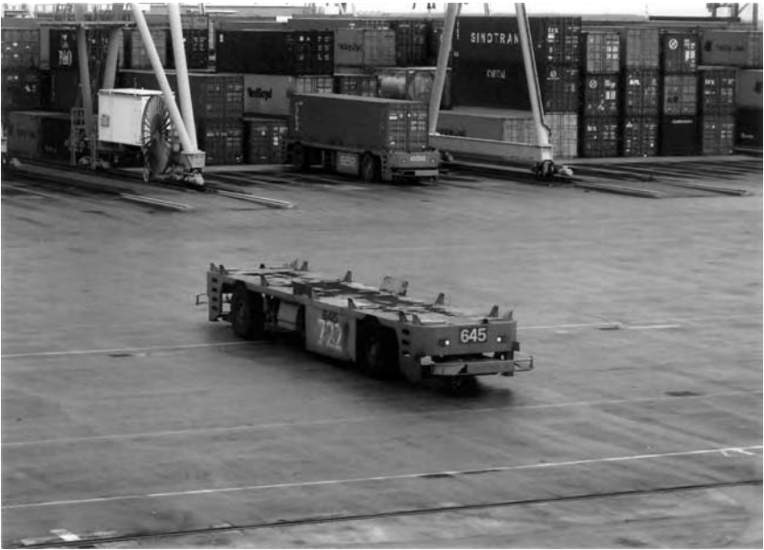
Fig. 8.29 Automated, driverless ground-handling transports deliver container units from the terminal stack to the underside of ship/shore gantry cranes.
