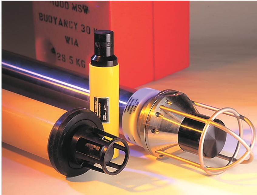
Figure 5 – Typical transponders used for surface and underwater position reference
