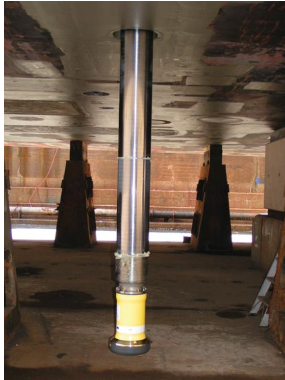
Figure 7 – An example of a transducer pole for installation through the hull
