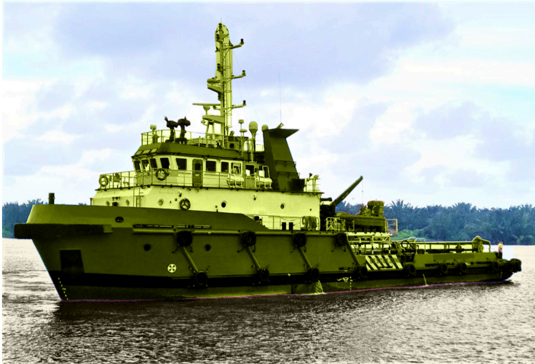
2008 | 40 M | 1/2 FIFI | 20 T BP | Utility Support Vessel
