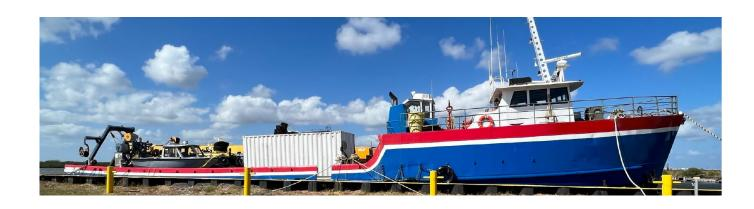
This U.S.-flagged offshore support vessel, with a gross tonnage of 99 tons and a length of 120 feet, has a 70 x 25 ft deck with a 100-ton load capacity. Powered by Detroit Diesel engines (1200 HP) and equipped with DP-1 dynamic positioning, it operates at 12 knots and accommodates up to 14 crew members. Designed for dive and survey support, the vessel includes a man-rated crane, launch and recovery system, fiberoptic winch, and a range of specialized survey equipment for offshore tasks.
