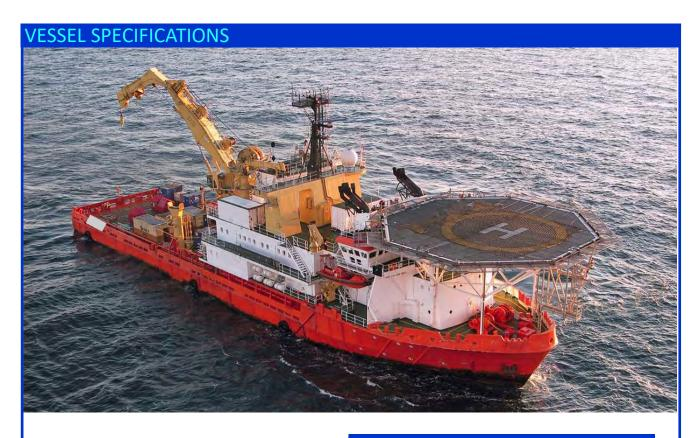
This 82M LOA UT705 Norwegian design Multi-purpose Offshore Construction, Diving Support and Accommodation Vessel track history has a proven Walk-to-Work, ROV support, Sat/ Air Diving scopes of work and multiple types of surveys globally. She is classed vessel with multi role capabilities for subsea and surface offshore operations.
