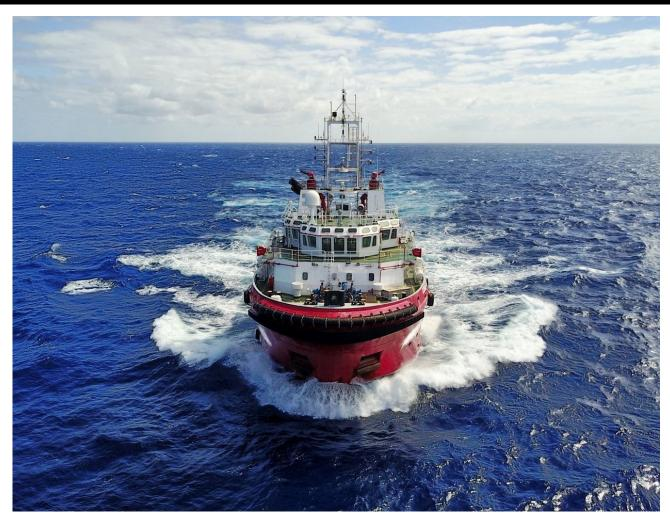
The anchor handling tug supply vessel is specially modified to serve as a dedicated emergency towage vessel (ETV). It is uniquely designed for emergency towage tasks, ready to respond to maritime casualties as directed.
