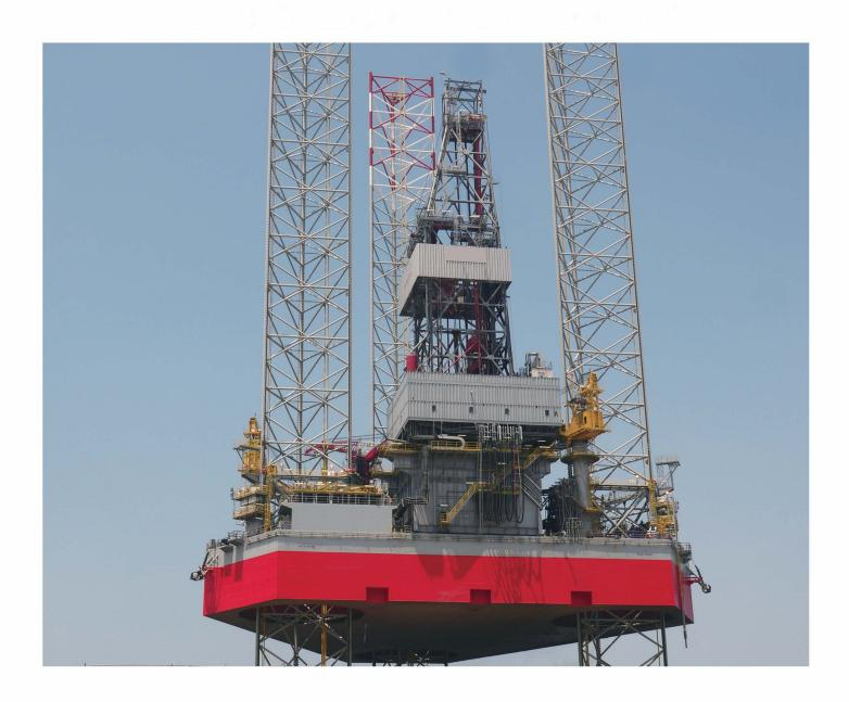
This Jack-up Drilling Rig is designed by an American design company - F&G. It is able to operate at water depth up to 120m (400ft) and drill wells down to 10668m (35000ft) at -20 C. It can be operated in an extreme harsh environment. Hot/ fit for work Jack-Up Rig.
