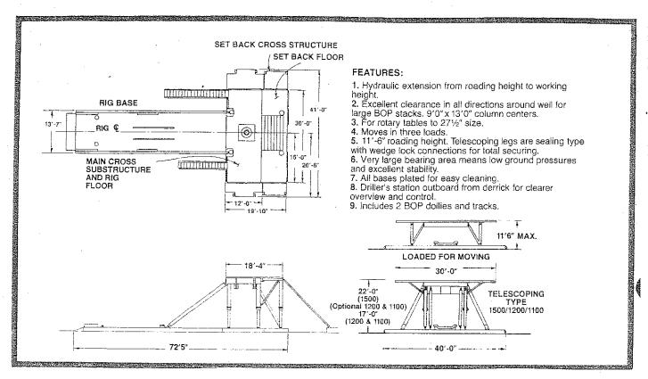
STACKED SUBSTRUCTURE WITH SETBACK CROSS BASE AND MAST CROSS BASE
