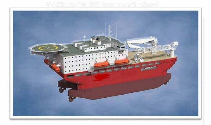
520Beds, - 38.5m +/- 8m Telescopic gangway - 100t NBC - Helideck to CAP 347 21,880 kW of power, 4 x 45 00 kW thrusters - Model Tank Tested Stable Platform ABS +A1 Mobile Offshore Unit, +AMS (E) DPS-3 UWILD, Helideck
