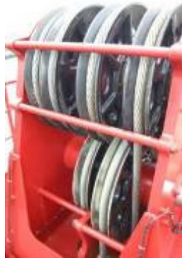
Figure 1: Head crane house with retaining bars (typical)
