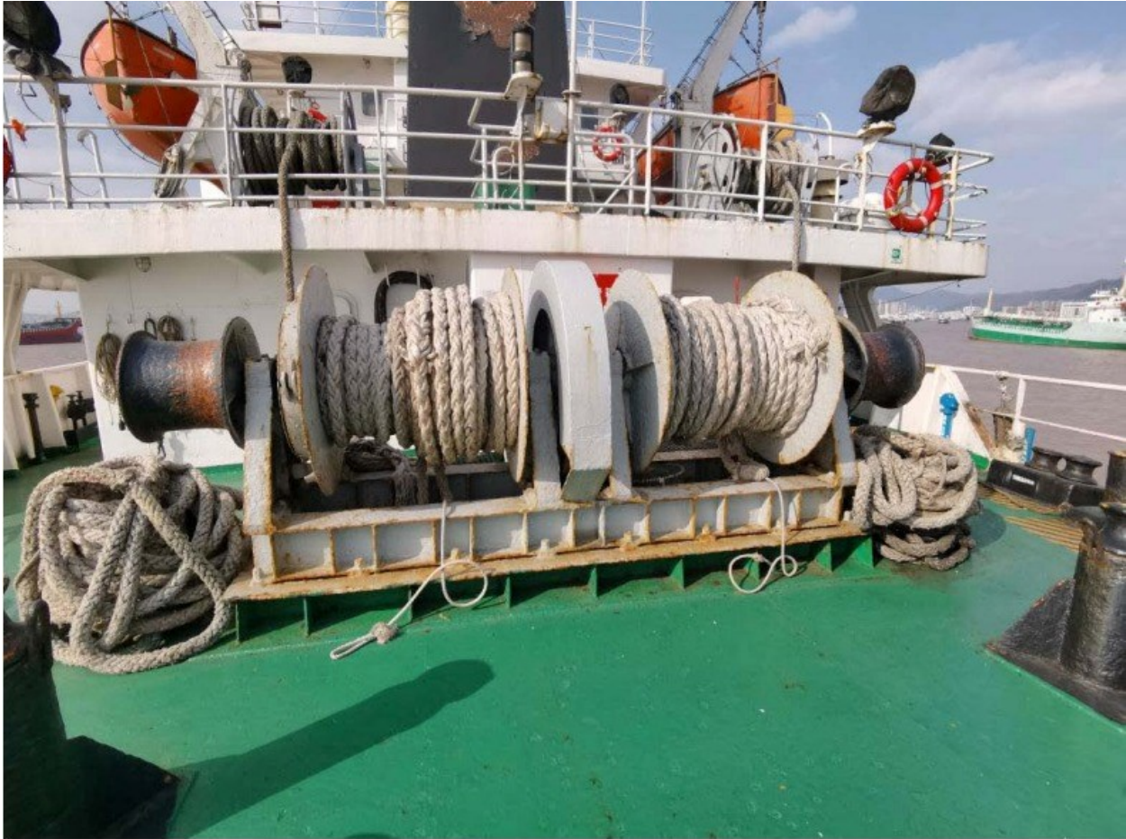
(22) Condition of mooring winch
