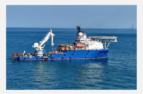
Dynamically Positioned (DP-2) Offshore Subsea Support Vessel, well equipped for offshore Construction, ROV, Diving, Survey and Geo-technical support roles. She is built in 2011, DNV Classed vessel and fully SPS compliant, with an overall length of 82 meters and breadth of 20m she provides over 700m<sup>2</sup> of clear deck space, 150sqm of mezzanine deck and over 1,000mt of cargo carrying capacity.
