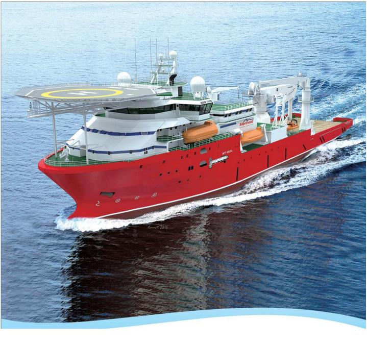
Built in 2017 this DP2 Multipurpose Specialized Diving Support Construction Vessel has an 18-man twin-bell Saturation Diving system, a 140T AHC offshore crane, SPS compliant and can accommodate up to 130 personnel.
